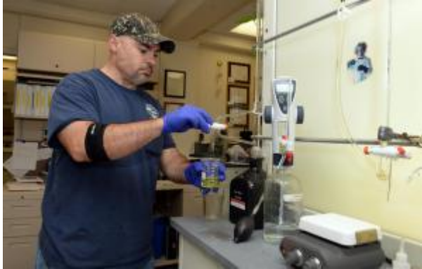
Steve Callahan, an operator at the Antioch water treatment plant, demonstrates how to perform a chloride titration test to determine the chloride level in water. (Susan Tripp Pollard/Bay Area News Group)
